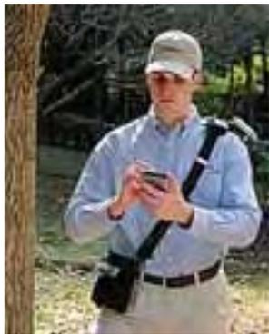
A surveyor records the location of an endangered tree using a Sokkia GIR1600 wearable GPS receiver and a PDA with geographic information systems software. Global positioning services are the most dynamic and visible applications of space infrastructure today. *Image Credit: Sokkia*
